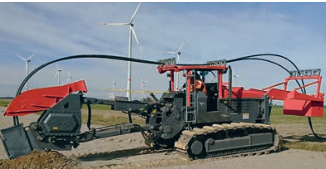
V225 with track pads for protection of paved surfaces
